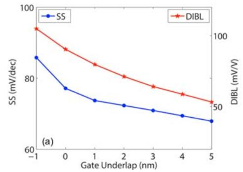
**Figure 3:** SS and DIBL in a DG UTB FET with  $L_G = 15$ nm as a function of the length of the gate underlap region  $L_{und}$ .  $L_{und} < 0$  indicates gate overlap instead of underlap.
