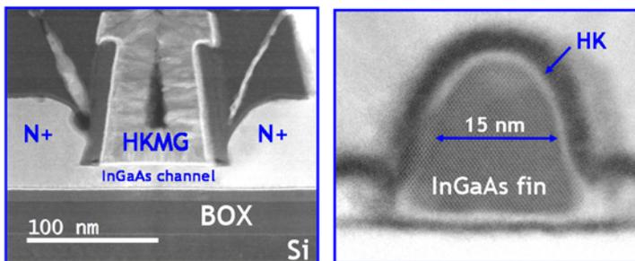
**Figure 4:** InGaAs UTB SOI and Fin MOSFETs
