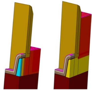
**Figure 7:** Realistic Silicon (left) and InGaAs (right) n-FinFETs used in TCAD simulations.  $L_G = 15 \text{ nm}$ ,  $H_{Fin} = 20 \text{ nm}$ ,  $W_{Top} = 5.5$ , taper angle =  $7^\circ$ . The InGaAs device has the same basic geometry as the Silicon one, but raised S/D and lowly doped n-type (instead of p-type) channel.
