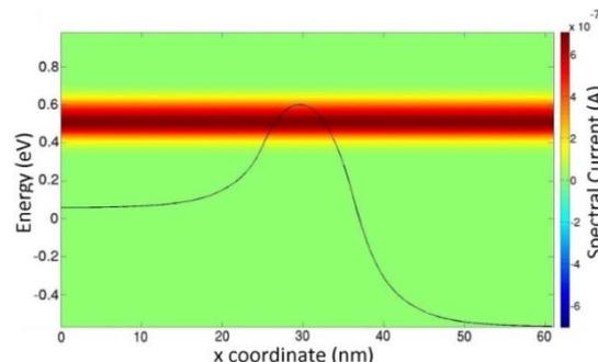
Figure 2: Spectral current in a double gate ultra-thin body (DG-UTB) FET with  $L_G = 10\text{nm}$  showing strong source-to-drain tunneling (SDT).
