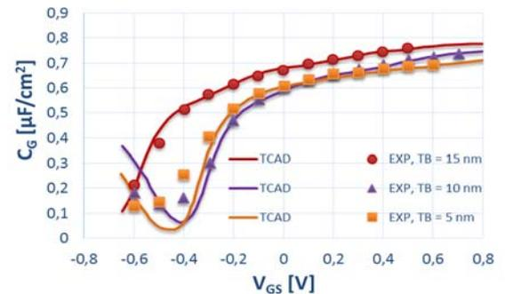
Figure 5: IMEC InGaAs MOSFETs CV curves
