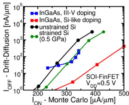
**Figure 8:**  $I_{OFF}-I_{ON}$  relation for Si and InGaAs n-FinFETs.
